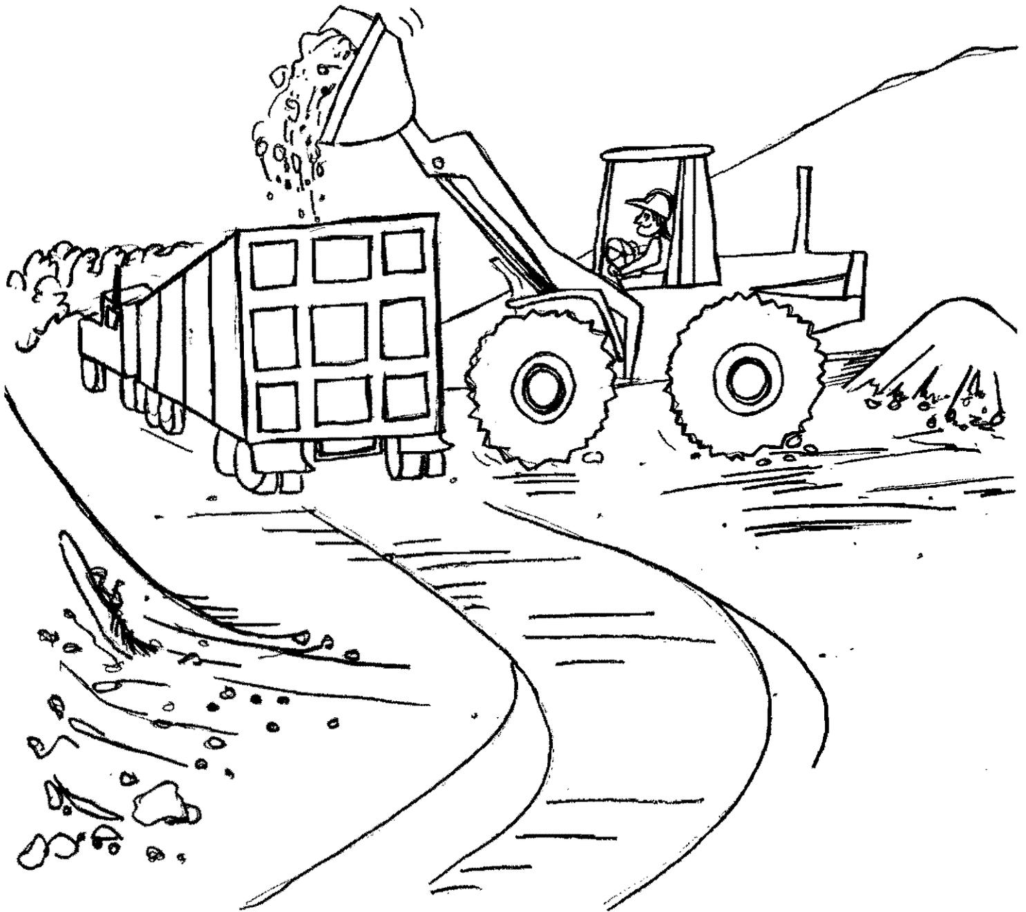
The mining, crushing and washing of the gravel takes place at the mine site. From the mine site, the gravel is loaded into big trucks and hauled to building sites or processing plants.
