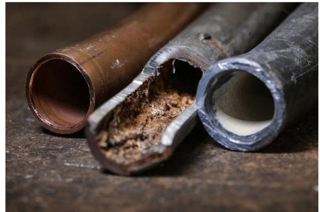
Three pipes (left to right): A copper pipe, a corroded lead pipe, and a lead pipe that has been treated with phosphate corrosion inhibitors to reduce the risk of lead leaching into the drinking water. Photo courtesy of Passaic Valley Water Commission.
