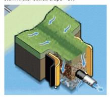
• French Drain- Underground pipe surrounded by gravel and landscape fabric that soaks water into ground until ground is full then carries water away in a pipe. Must be protected from aggressive tree roots.
