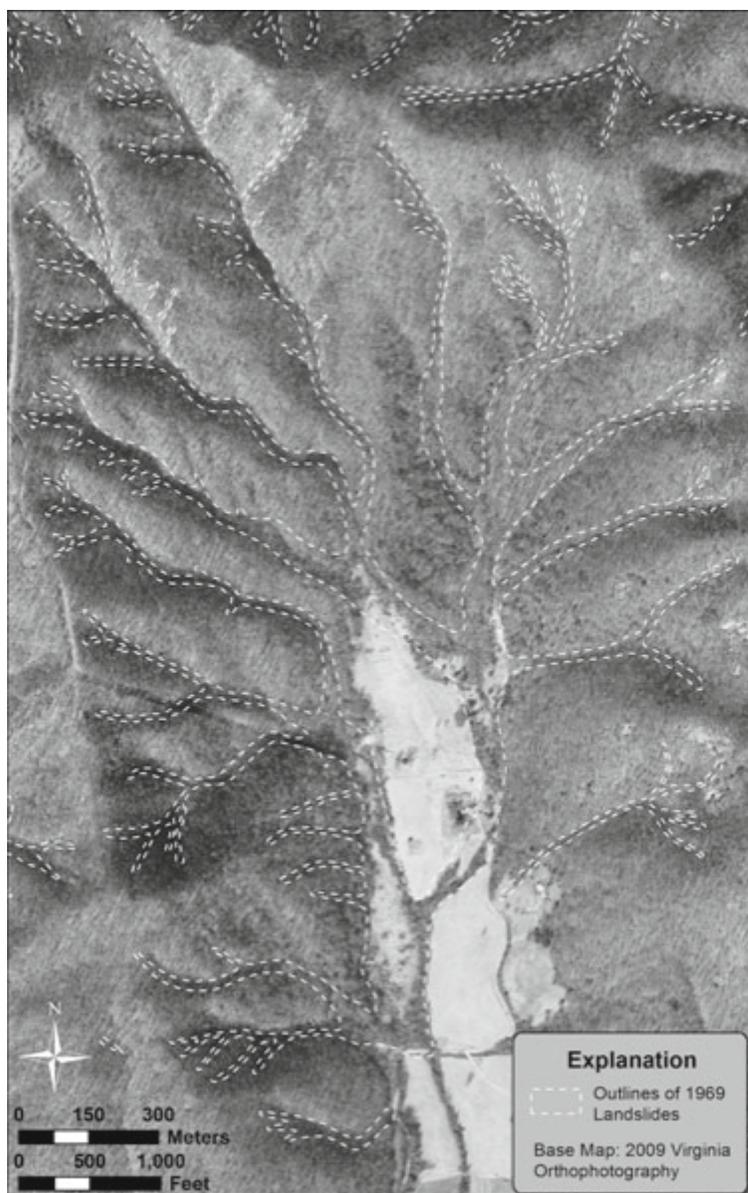
Figure 3 Outlines of 1969 landslides in Fortunes Cove area of Nelson County illustrate typical debris flow “sources” or origination points.<sup>9</sup>
